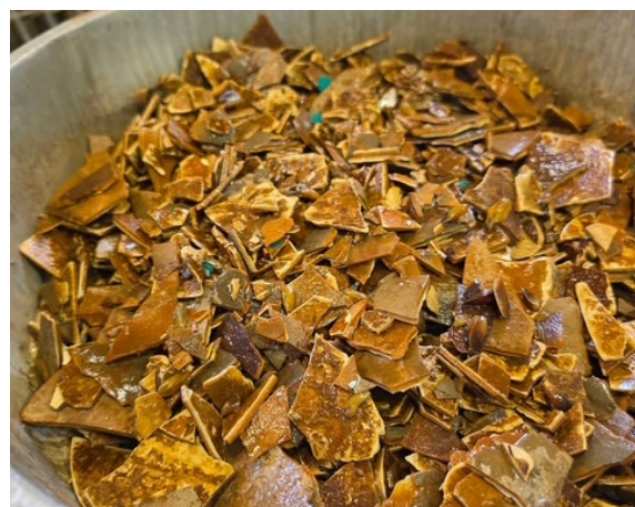
Scale from Heat Exchanger – PP4
